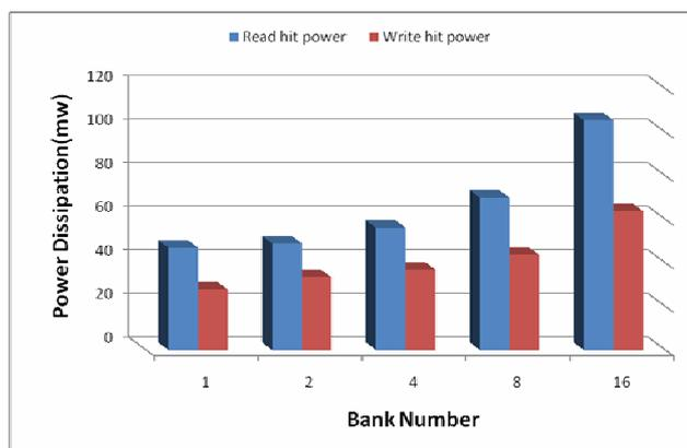
**Figure 7:** Read and write hitt power results for various cache's bank number.
